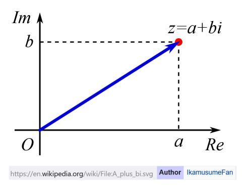
Length of the blue arrow (distance of the z number from the origin) is the so called modulus ("length") of a complex number, which is calculated as:
